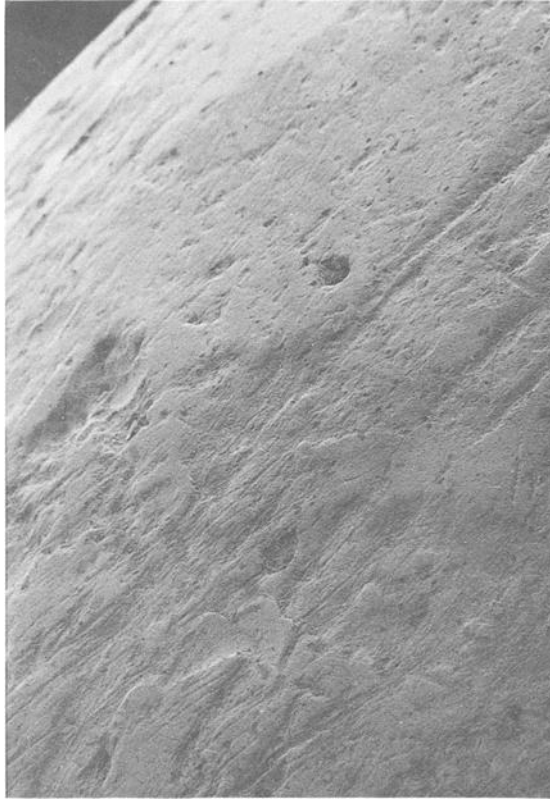
FIG. 4— Surface of non-deformed shot (original magnification, \times 30 ).
